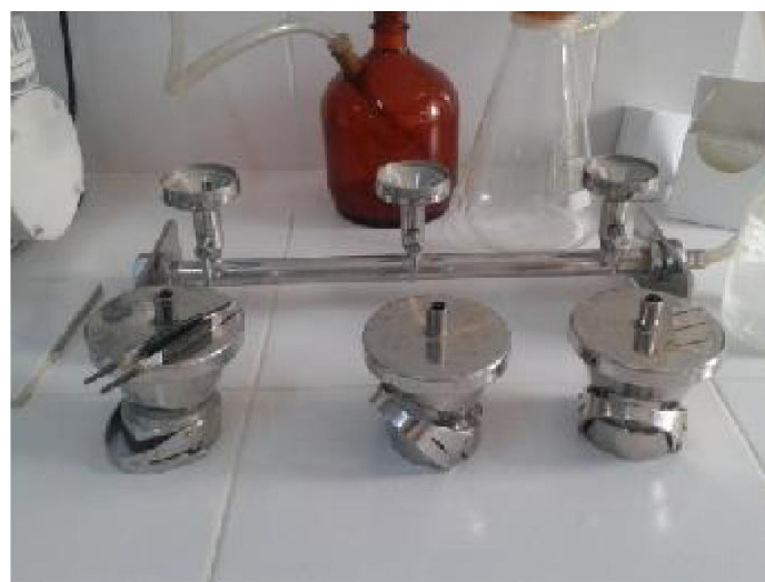
Rampe a filtration
