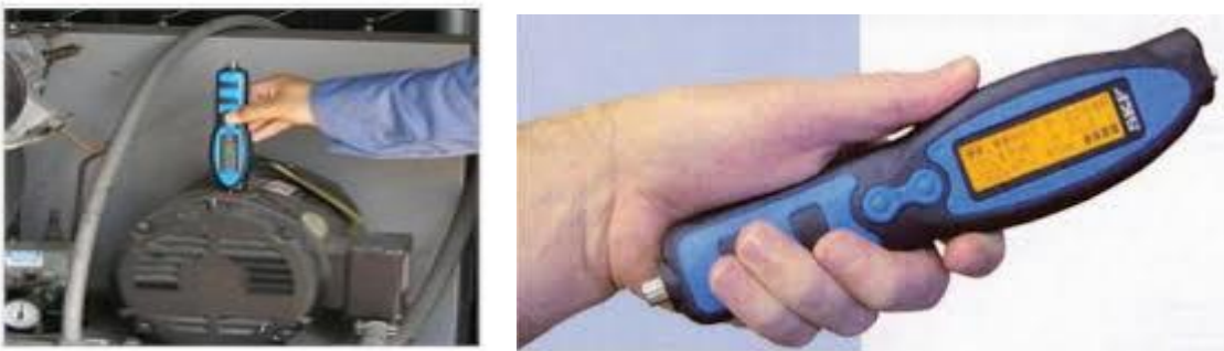
Figure 38 :le SKF Machine Condition Advisor.
