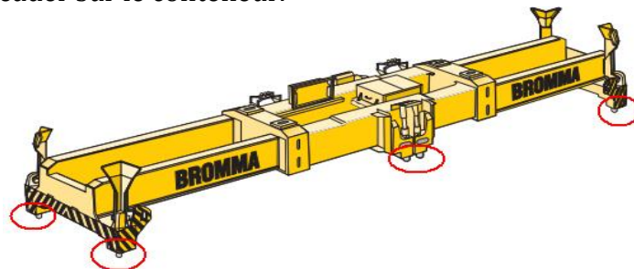
Figure 15 : Emplacement des twists locks
