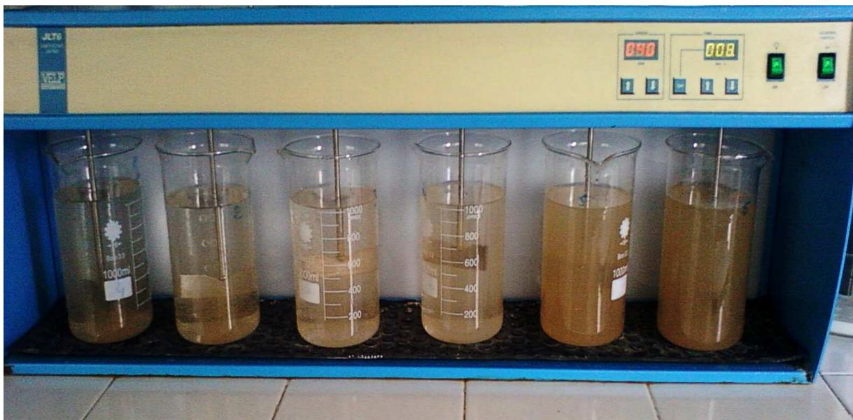
**Figure 11: essai de coagulation-floculation**
