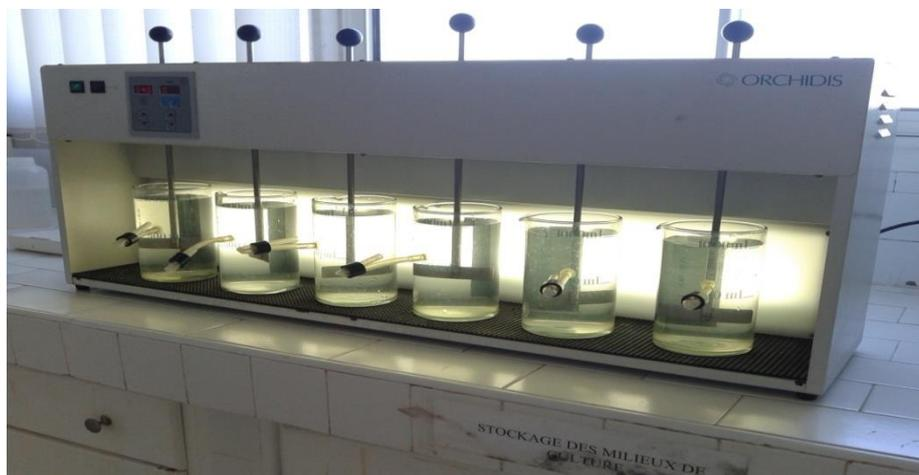
**Figure 9: Appareil jar-test**
