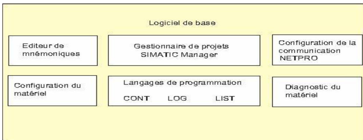
Figure 15: ARCHITECTURE DE CONSTRUCTION D'UN S7 400.
