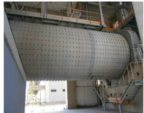
*Figure I.15: Broyeur ciment*
