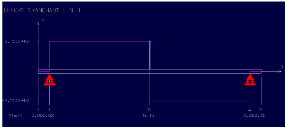
Figure 5.2: Diagramme des efforts tranchants
