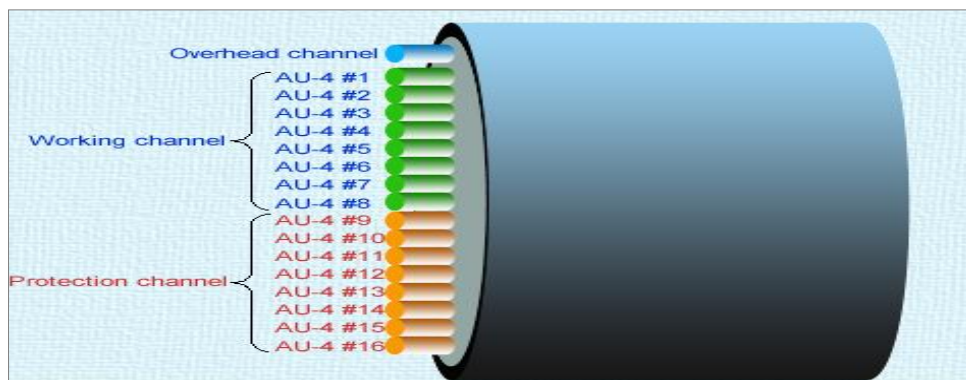
Figure 38 : MSP Ring's working and protection channels.
