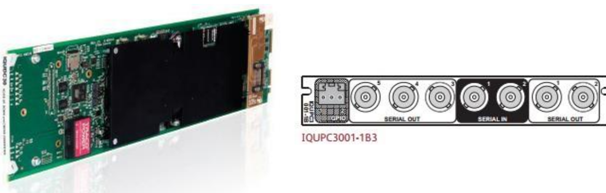
Figure 34 : SDI Up-converter IQUPC30 de Snell Group [15]
