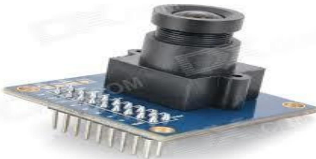
Figure 13: Module camera OV7670
