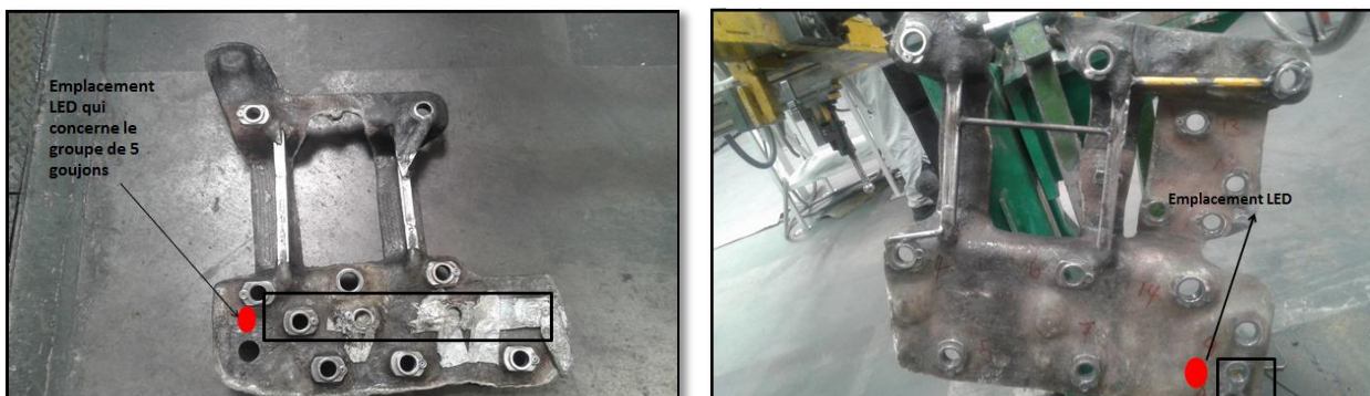
Figure 52: emplacement des leds
