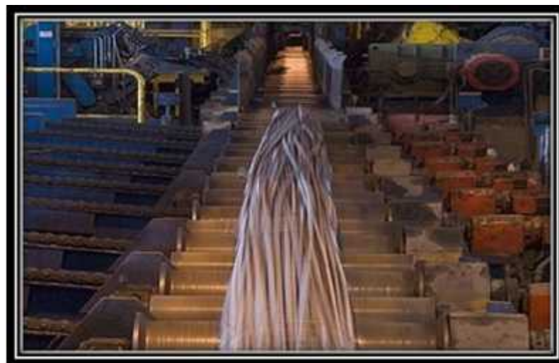
Figure 2 Zone de finissage
