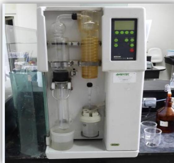
Figure 2:Appareil de distillation BUCHI.
