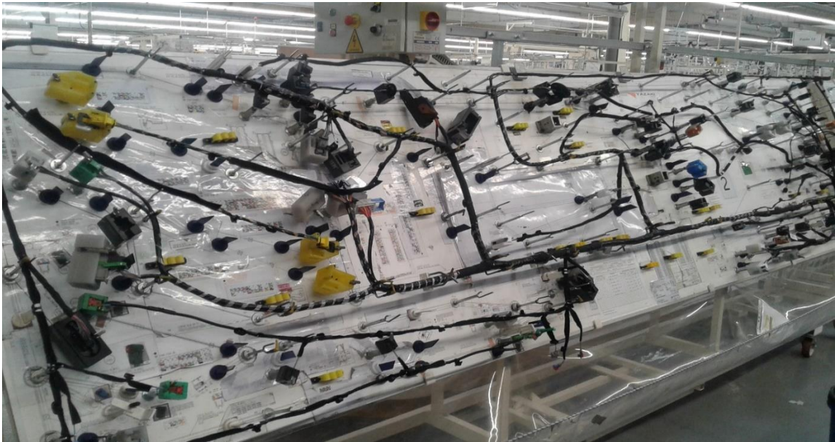
Figure 15 Assemblage câble ‘enrubannage’
