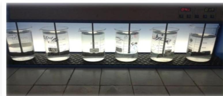
Figure 16: Appareil Jar Test
