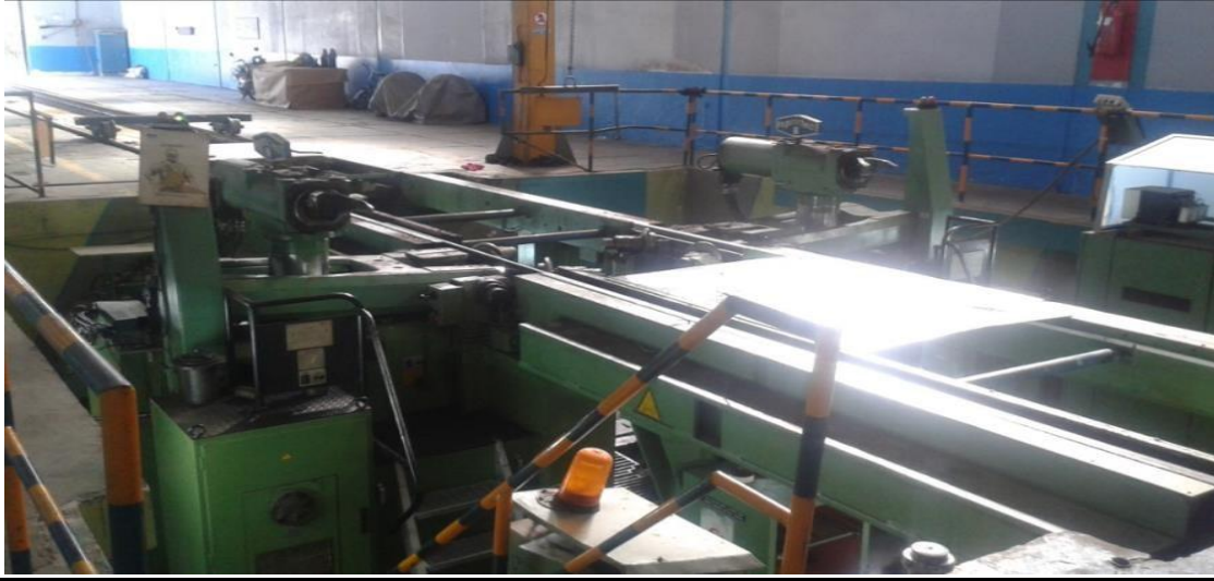
FIGURE 2.2: MACHINE TOUR CNC EN FOSSE
