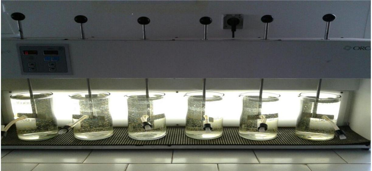
Figure 8: Appareil de jar-test
