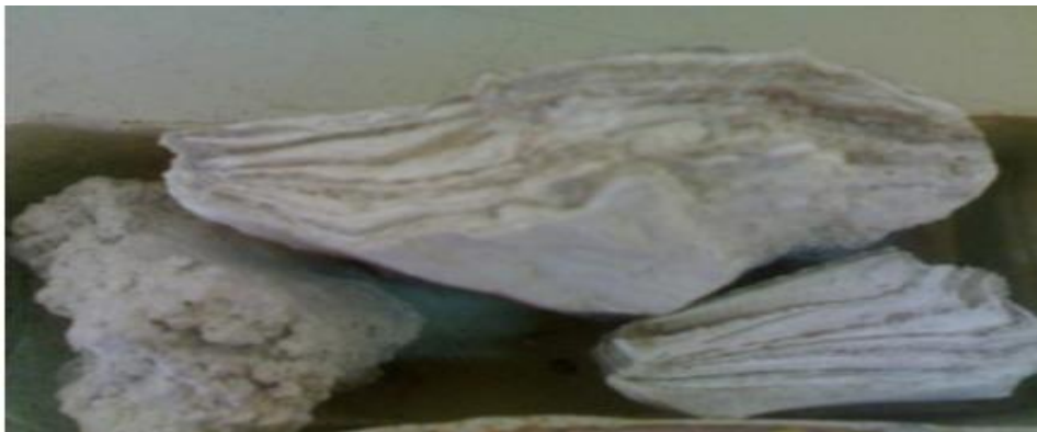
Figure 10 : Croute causant un bouchage
