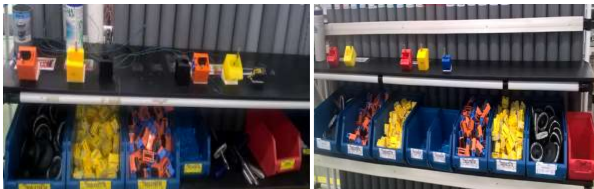
Figure 35: Two Bin System de Poste 12
