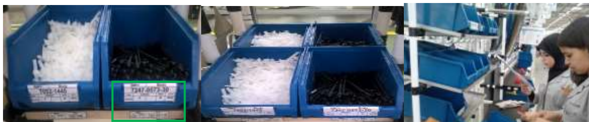
Figure 36: Mise en place de Two Bin System
