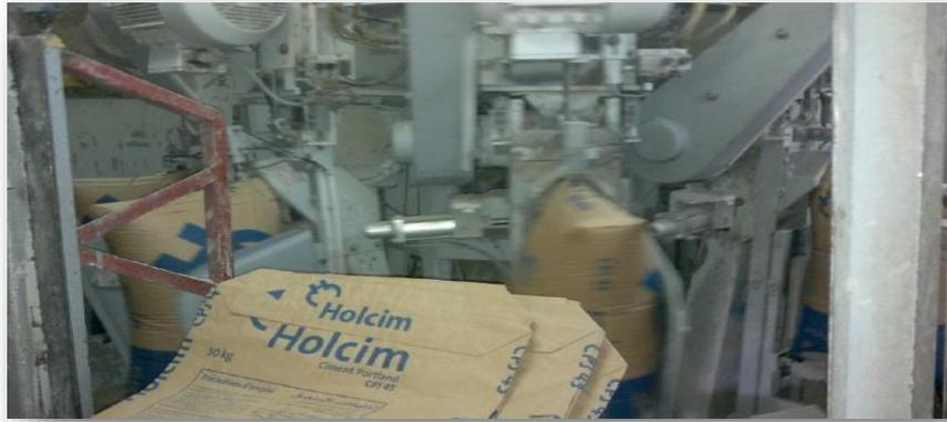
Figure 18: Ensacheuse rotative.
