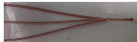
Figure 19: Joint simple End splice
