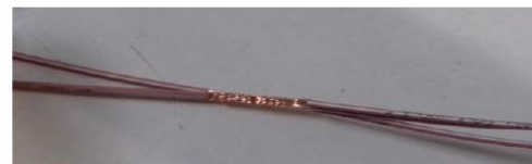
Figure 20: Joint simple Trough splice
