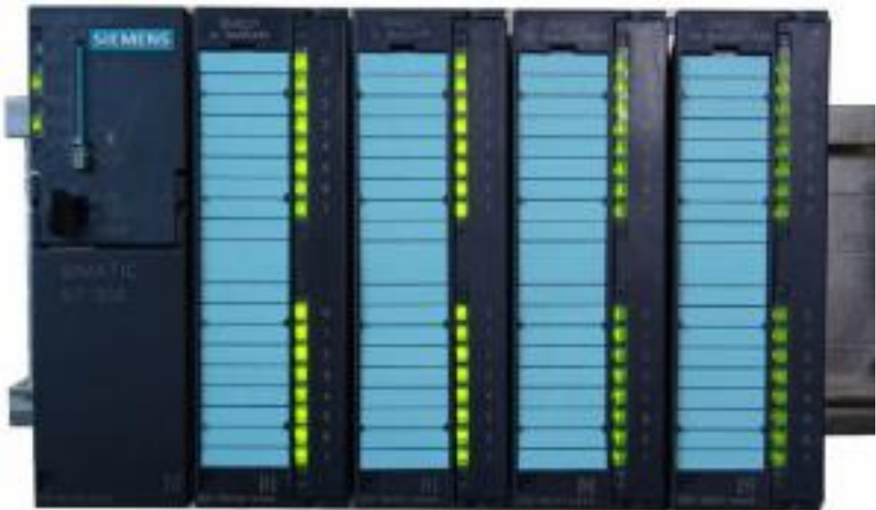
Figure 9 : Station Simatic s7-300 (CPU+ des module E/S)
