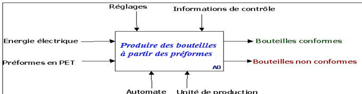
Figure 9: Diagramme SADT niveau A-0
