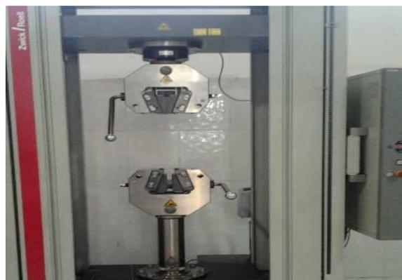
**Figure18:** Machine traction de 150 N
