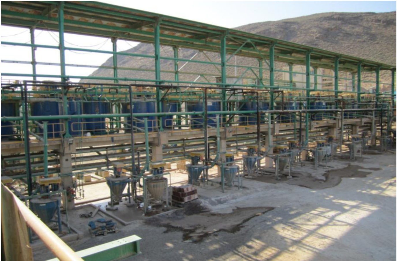
Figure II.6 : Montrant les cellules de flottation.
