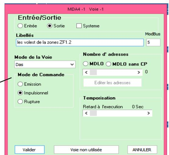
FIGURE 3.22- L'INTERFACE DECONFIGURATION D'UN VOIE DE MDA4.
