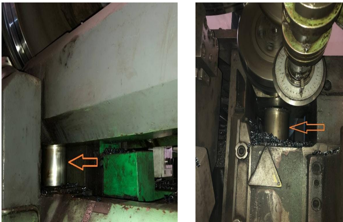
Figure 25: vérin (translation verticale des galets)
