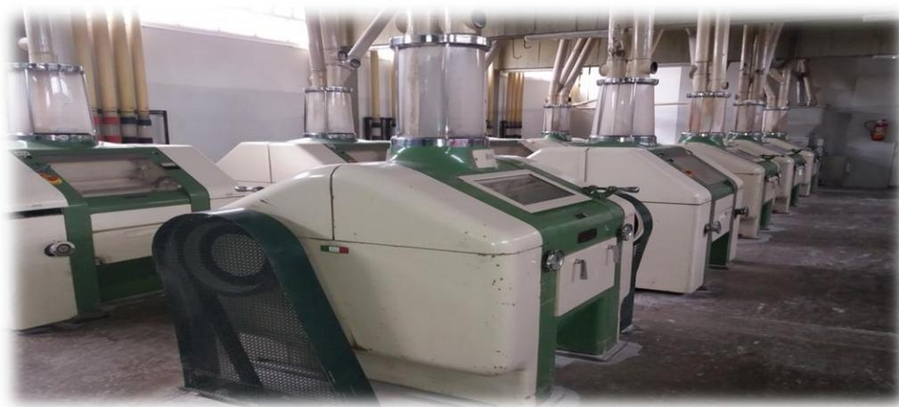
Figure 6: Appareils cylindriques
