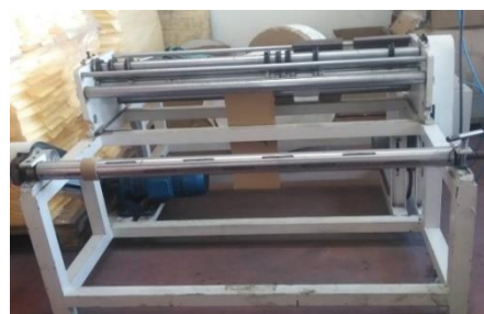
Figure 33: Machine de refendage.
