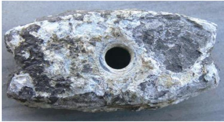
FIGURE 27: ANODE SACRIFICIELLE
