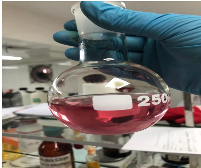
Figure 15: Zone de virage de dosage.
