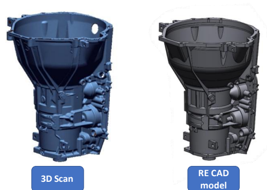
Figure 60: 3D scan vs CAD model. (Creaform)
