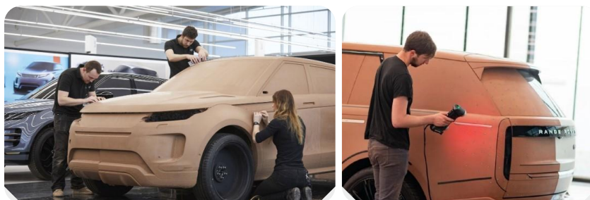
Figure 2: Using Creaform HandySCAN 3D to capture style of Range Rover.
