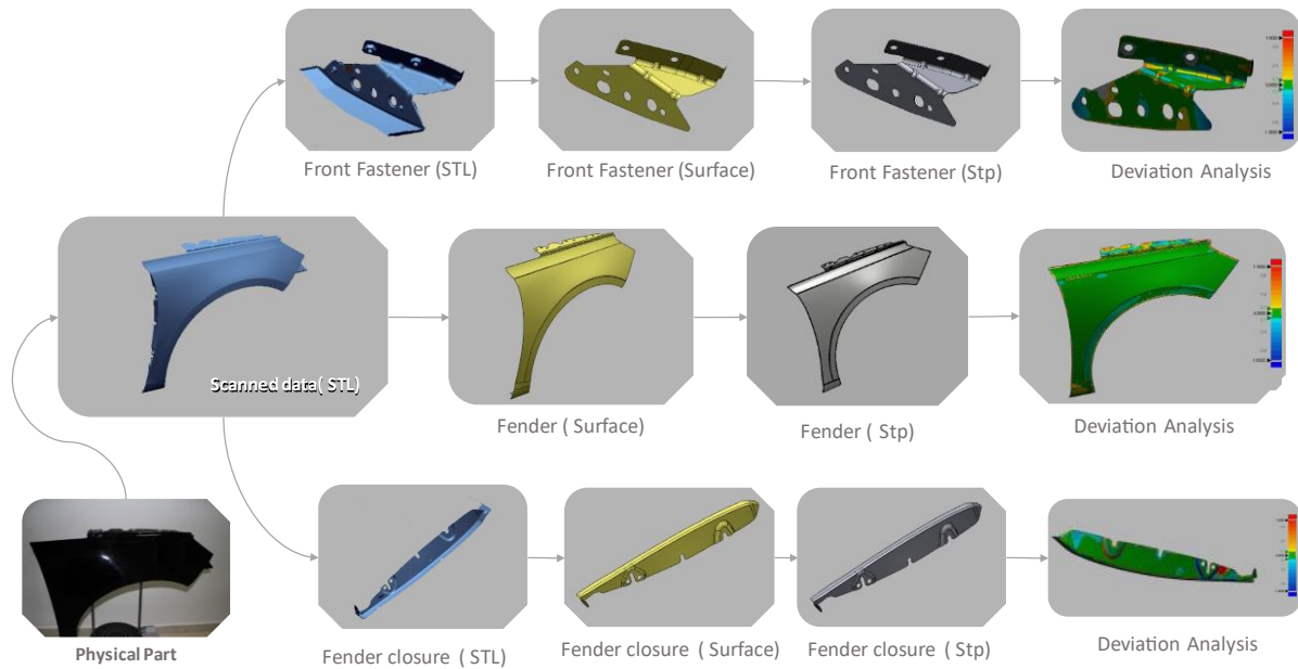
Figure 113: RE of all parts of the fender.
