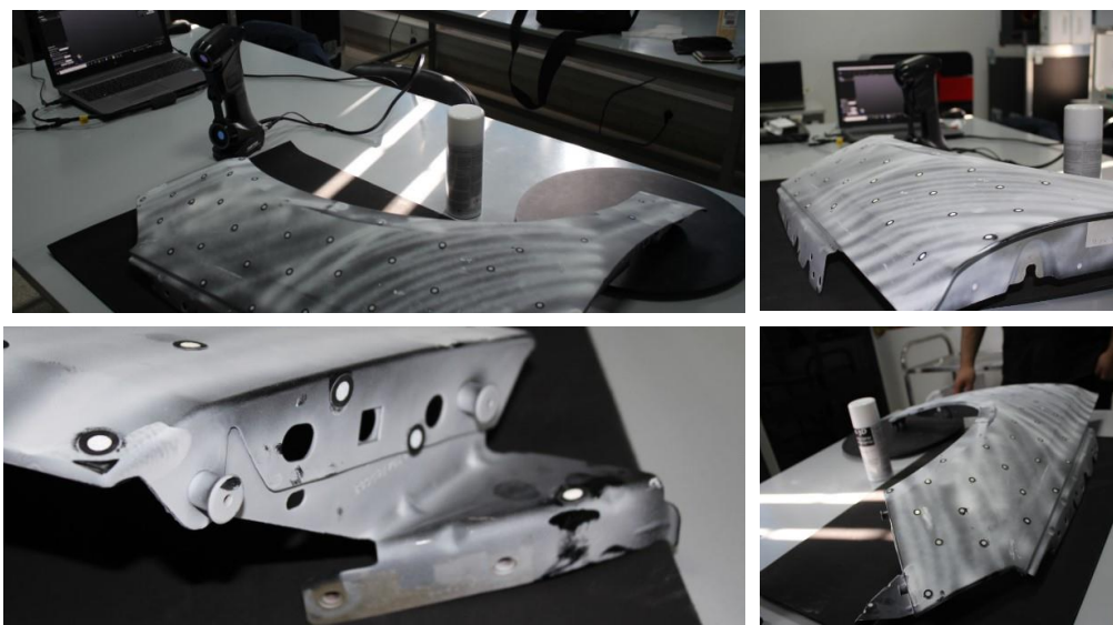
Figure 104: The sprayed fender with targets.
