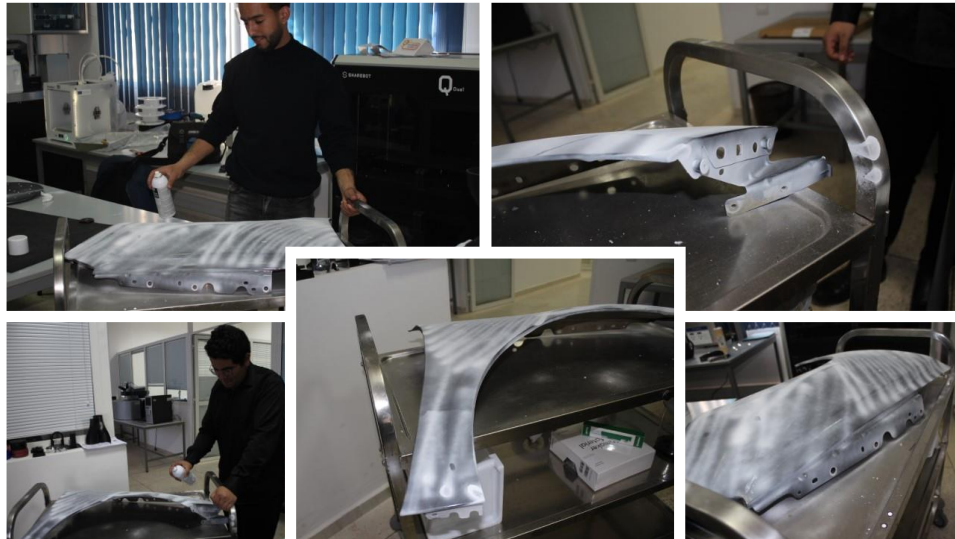
Figure 103: Spraying the fender with healing spray.
