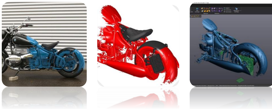
Figure 63: The use of HandySCAN 3d for production of prototypes and samples of custom bike accessories. (Abm motorradteile)
