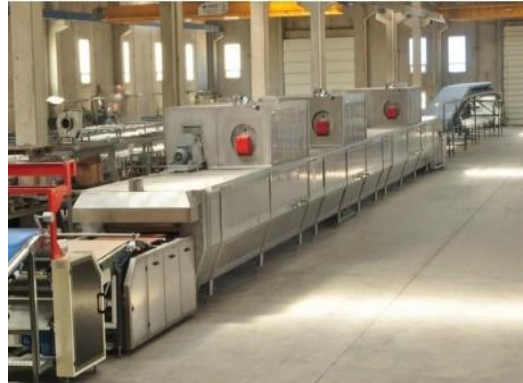
Figure 8 : Four tunnel de biscuit [8]
