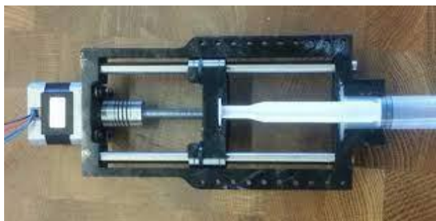
figure 25: extrudeuse de seringue
