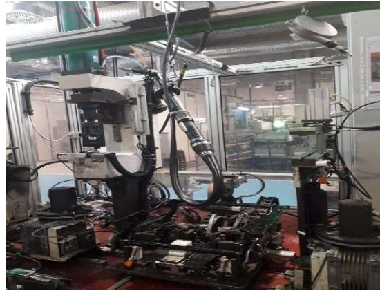
Figure 20 : operation de vissage
