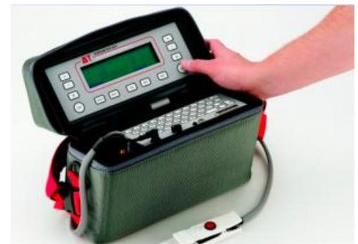
**Figure 9 :** POROMETRE de model AP4
