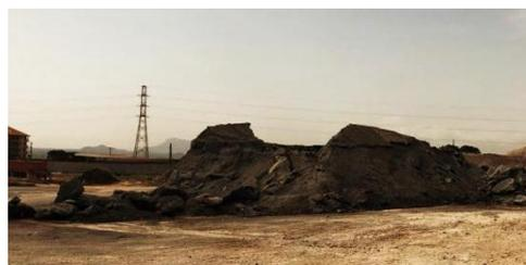
Figure 7: Laitier de Haut Fourneau
